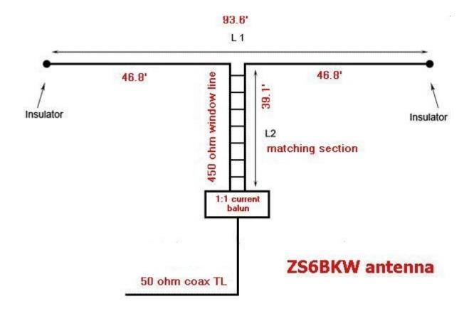
In the original design, 300 ohm twin was used, but I prefer the 450 ohm stuff. It's much stronger - and losses, especially in wet weather, are lower when impedances are high down the line. Back in 1985, 450 twin wasn't readily available, there was only 75 and 300 twin, or the option of making your own openwire feeders (which actually are the best of all – around 600 ohm, but these do tend to twist or get caught in trees etc! Yes – bitter experience and soldered joints here too!)
